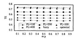
Figure 11. The comparison of TE with and without fuzzy controller under different moving probabilities.
