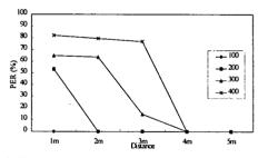
Figure 2. The measurement results of PER in different packet length under different distance.
