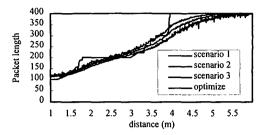
Figure 8. The adapted packet length obtained by PLFC at each distance under different simulation scenarios.
